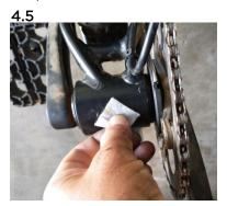
4.6 Remove the backing from the adhesive on the PAS sensor (#3). Rotate the crank so that the zip tie is inline with the sensor. Align the PAS sensor so that the face is parallel with the disc surface and there is about a 1/16 inch gap between the zip tie and sensor. You can use a credit card to establish the gap. Press down on the PAS sensor to adhere it to the bottom bracket. Apply additional pressure for about 30 seconds to fully activate the adhesive.
