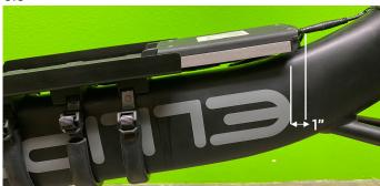
5.6 Connect the PAS and Motor extension cables to the controller. Adjust the controller position to eliminate cable slack.
