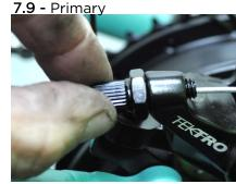
Caliper Barrel Adjuster
