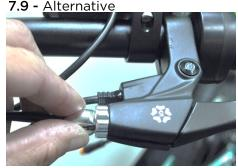
Brake Lever Barrel Adjuster
