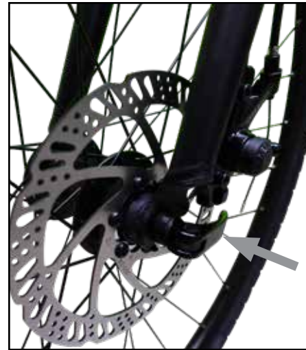
Left: Location of quick release lever on front wheel.
