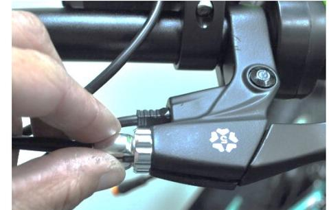
Brake Lever Barrel Adjuster
