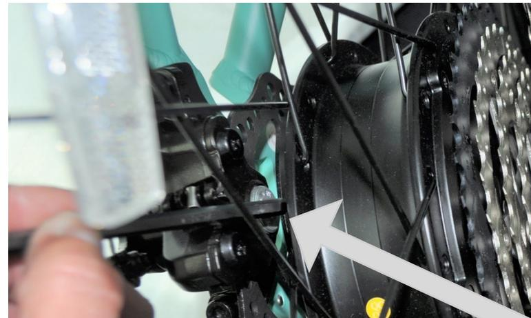
Brake Adjustment Wrench inserted in Adjustment Screw
