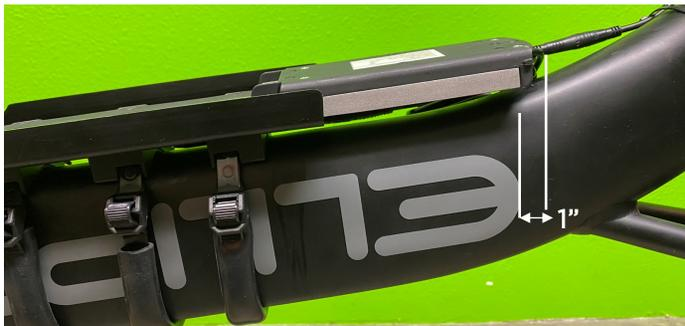
5.6 Connect the PAS and Motor extension cables to the controller. Adjust the controller position to eliminate cable slack.
