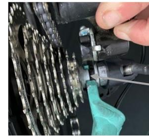
Non-Turn Washer Tab Oriented Down (View from Underneath)
