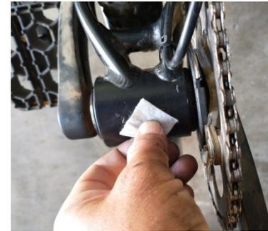
4.6 Remove the backing from the adhesive on the PAS sensor (#3). Rotate the crank so that the zip tie is in line with the sensor. Align the PAS sensor so that the face is parallel with the disc surface and there is about a 1/16 inch gap between the zip tie and sensor. You can use a credit card to establish the gap. Press down on the PAS sensor to adhere it to the bottom bracket. Apply additional pressure for about 30 seconds to fully activate the adhesive.
