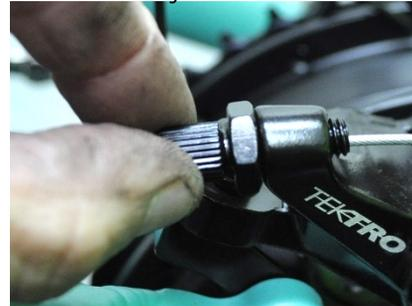
Caliper Barrel Adjuster
