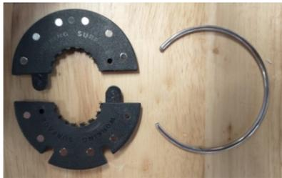
4.3 Install the PAS magnet disc on the right crank. Make sure the face of the disc labeled “working surface” (A) is facing inward toward the bike frame. Press the two pieces together. Install the retaining ring back around the disc. If the two pieces do not fully seat together, that is OK, the retaining ring will keep them together.
