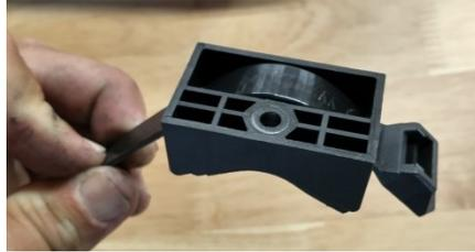
5.3 Using a 3mm Allen key, attach the battery cover (#17) to the controller with the three battery bracket screws (#10) and then use the screws to attach the three brackets. Tighten to 5 N-m.
