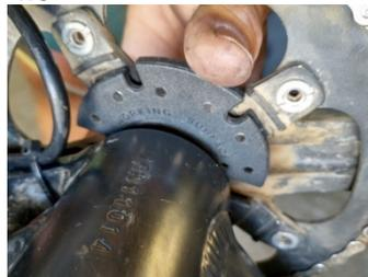
4.4 Secure the magnet disc to one of the legs of the crank spider using a small zip tie. Make sure the head of the zip tie sits on the outside of the crank spider, away from the bike. Trim off the excess zip tie.
