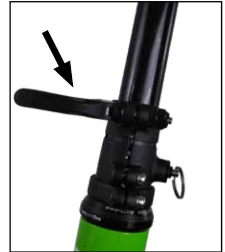
Right: Location of quick release lever on steering column.
