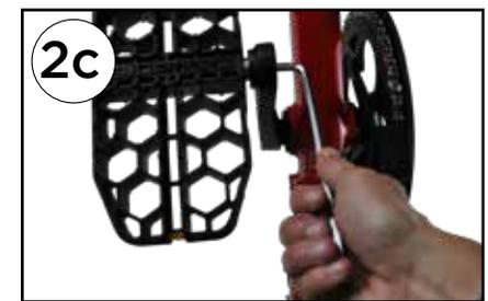
3. Insert the left retention screw into the left pedal axle. Use the 4mm Allen key to tighten it by rotating it clockwise (when facing the head of the screw) until it is fully-seated and torqued to 6 Nm.
