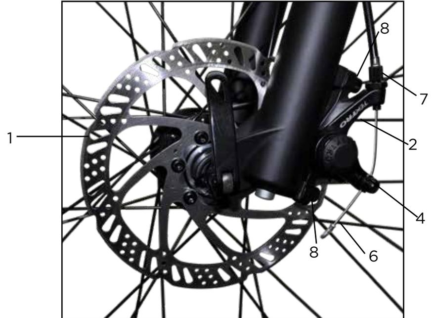
**▲WARNING!** Ensure that the brake quick release system is properly closed and your brakes are functioning properly before riding your bike. If the brake quick release system is open or closed improperly, the brake will not function. Riding without operating brakes is extremely dangerous and drastically increases the likelihood that the rider will collide with another object and suffer serious injury.
