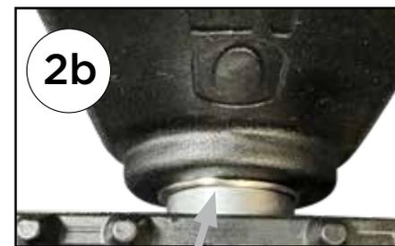
Improper Washer Install
