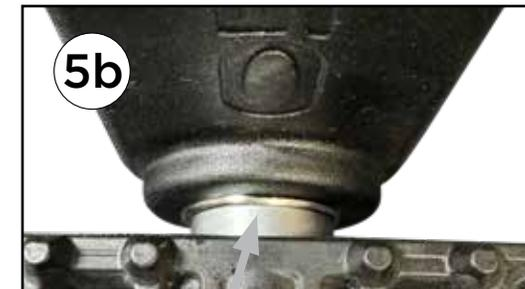
Improper Washer Install
