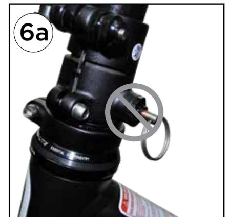
**⚠️WARNING! THE SAFETY INDEX PIN SHOULD BE FULLY SEATED SO THAT NO RED MARKINGS ARE VISIBLE ONCE THE STEERING HEIGHT IS SET. Failure to fully seat the index pin could result in the steering column collapsing during operation. This would likely cause the rider to lose control and fall.**
