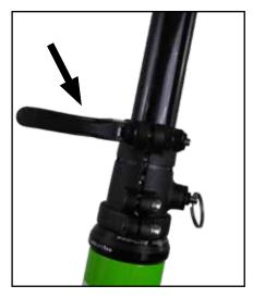
Right: Location of quick release lever on steering column.
