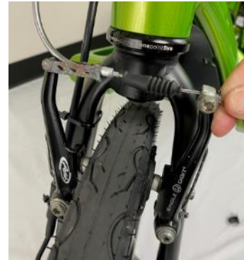
Pull brake cable tight
