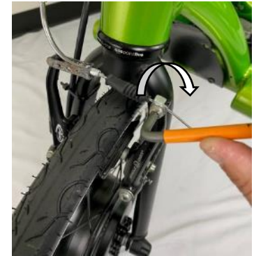
Tighten cable pinch bolt
