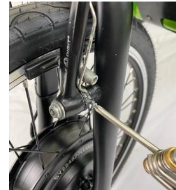
Tighten cable pinch bolt
